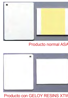
◆ Reg. ASA Xenon ● Reg. ASA Arizona ▲ XTWE270 Xenon ▲ XTWE270 Arizona *2500 kJ/m² G26 Xenon Arc - 1 year Outdoor weathering
